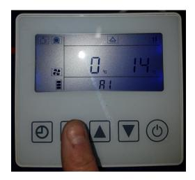
The up and down keys can now be used to view the status of all sensors.
